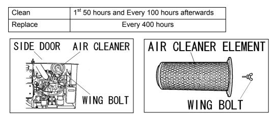
Loosen the wing bolts in the air cleaner and remove the air element. Clean or replace the air element.
